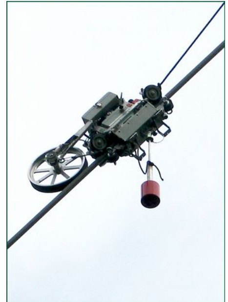
testing a guy rope of a transmitter via WLAN
